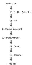
To stop a countdown operation, first pause it and then press (E). This will reset the timer to its start time.
