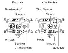
\* [F] is displayed for the final time number when an elapsed time measurement operation is stopped.
