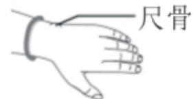
5.2 Closely attach the heart rate sensor to the skin with well contact in measurement of heart rate. The sensor light will expose if the smart bracelet is too loose, which will cause inaccurate measurement values. DO NOT directly look at the green light of the sensor in case that your eyes feel uncomfortable.
